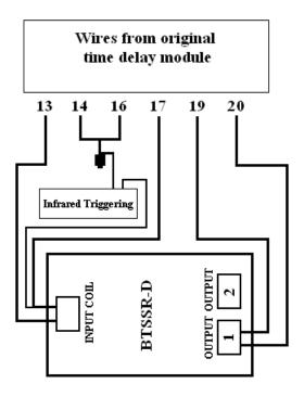
Replacing the Time Delay Module with the BTSSR-D
